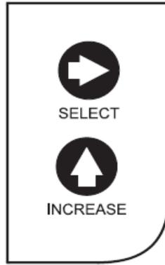
23. This will clear the SR-260 message and the display should now display 000.000. If an Error Code appears, record the value and depress the SELECT button until the display has the 000.000 view.
